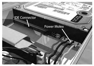
3) Using the included screws (larger ones), screw the hard drive onto the case through the holes on the bottom of the body (see image below).
